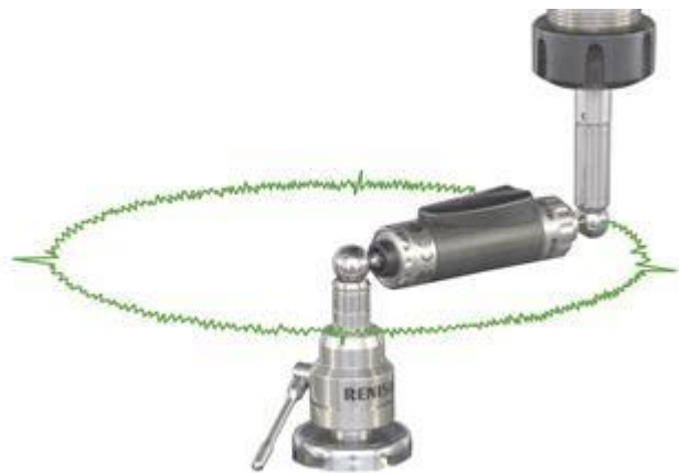
Measurement with Ballbar
